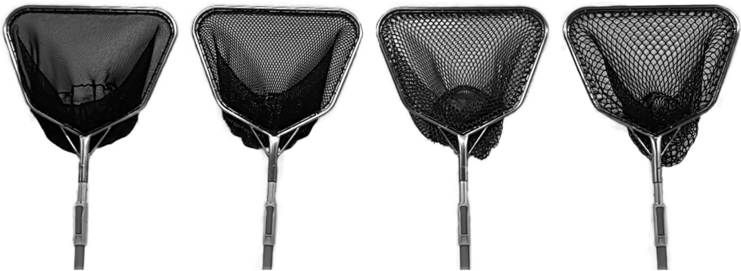
Figure 1. Dip nets with pentagonal frames ( 55 \text{ cm} \times 40 \text{ cm} ) and mesh sizes of (from the left) 5, 10, 15, and 20 mm, respectively.
