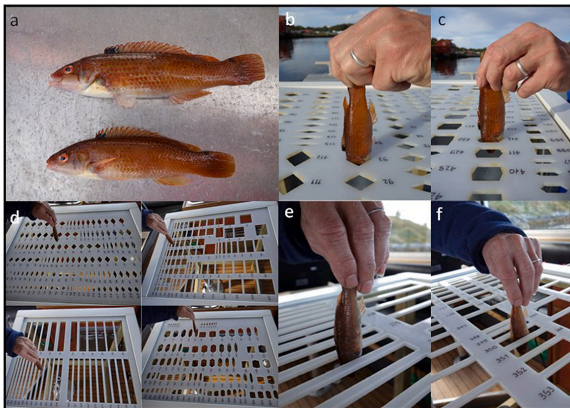
Fig. 3. Photo (a) shows a sample of two goldsinny wrasse used in the fall-through tests, (b-c) and (e-f) illustrate the fall-through procedure for different shaped openings, and (d) shows the different templates employed in the fall-through tests.
