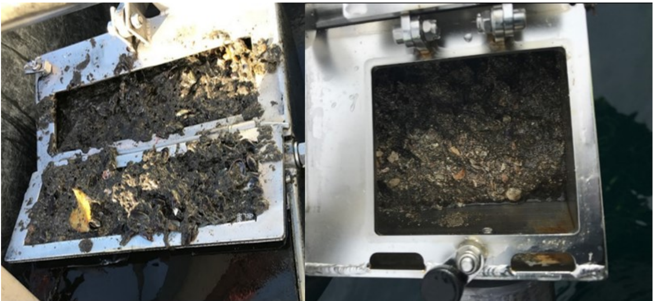
Figure 4. Grab haul with sediments from an Active aquaculture area (left) and shell sand from Non-active aquaculture area (right).
