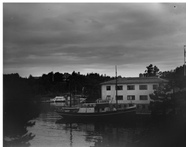
Figure 3. R/V Johan Hjort (2). Johan Hjort (2) was launched in 1931 with the aim to support the fisheries in a period of economic depression. The small ship operated mainly in coastal waters but was the first Norwegian vessel equipped with an echo-sounder (Schwach, 2004; Havforskningsinstituttet, 2008). Technical specifications: Shipyard: Gravdal Skipsbyggeri, Norway; built, 1932; length, 80 ft (25 m.); beam (not known); grt., 67 brt; main machinery, 90–120 hp (66–88 kw). Illustration: Courtesy of Institute of Marine Research.
