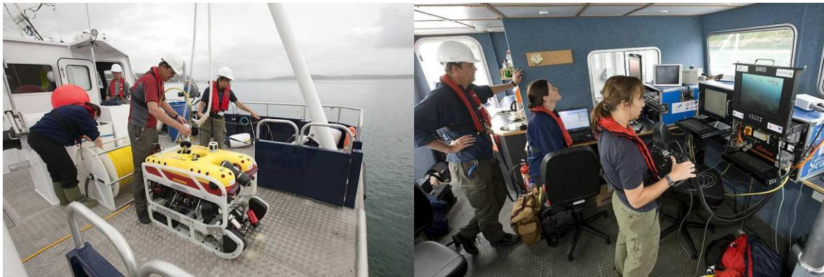
Plate 1 The launch and operation of the Seaeye Falcon ROV from the RV Falcon Spirit.
