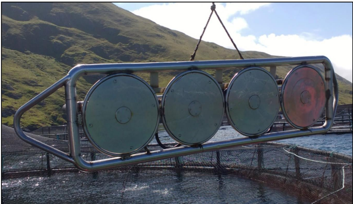
Figure 2.2.3-1. Example of a net cleaning rig from AKVA with 4 cleaning heads. Photograph courtesy of N. Ribeiro, with permission.
