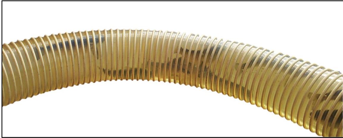
Figure 1.2-3. The behaviour of fish during pumping can be monitored through a transparent hose. Photo: Å. M. Espmark
