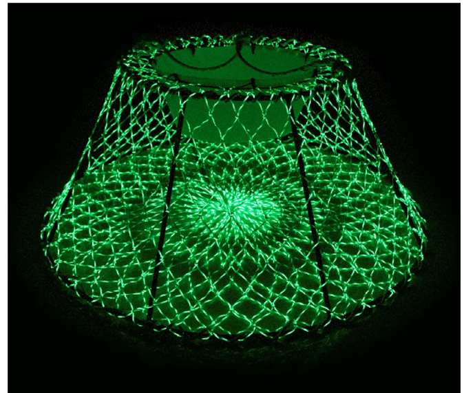
FIGURE 2. A photograph of an experimental luminescent trap in the dark.
