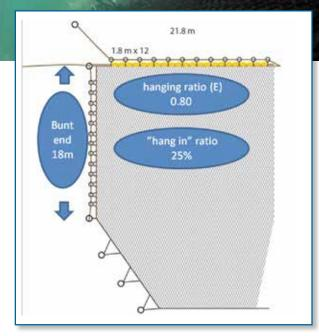
**Figure 1:** Proposed rigging for the codend/extension of purse seines in keeping with "best practices" for the release of fish from purse seines: Stretched length of the bunt-end should be at least 18 m; the minimum hanging ratio (E) of the bunt netting should be 0.8 or alternatively the maximum "hang in" of the meshes should be 25%.
