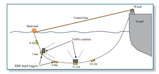
**Figure 2:** To document the release opening shape and to observe fish behaviour during release, depth sensors and GoPro video cameras were placed on the codend/extension.
