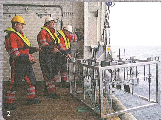
2. The multicorer samples the sediments without destroying the layers and surface structures. With this gear geologists and chemists can describe time series of changes in deposition of natural as well as anthropogenic chemical components.
