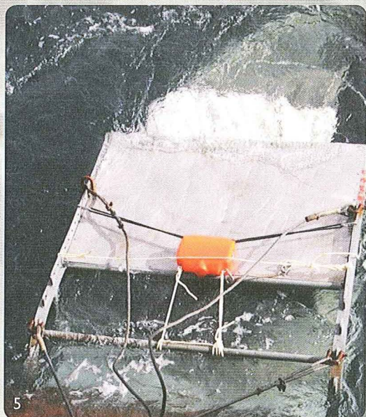
3. Larger epifauna are best collected with a small epibenthic trawl. MAREANO uses a 2 m wide beam trawl for this purpose. The specimens collected are valuable as ground truthing of species observed on the video.
