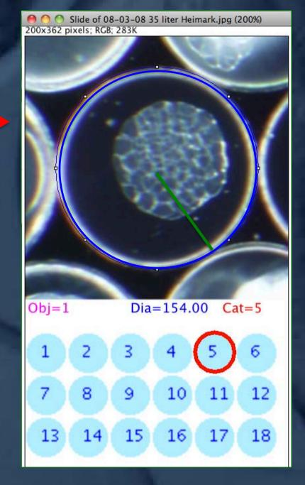
Slide show: The automatically measured diameter can be adjusted and the egg can be assigned a category. Category is displayed using a hand of a clock analogy (green line).
