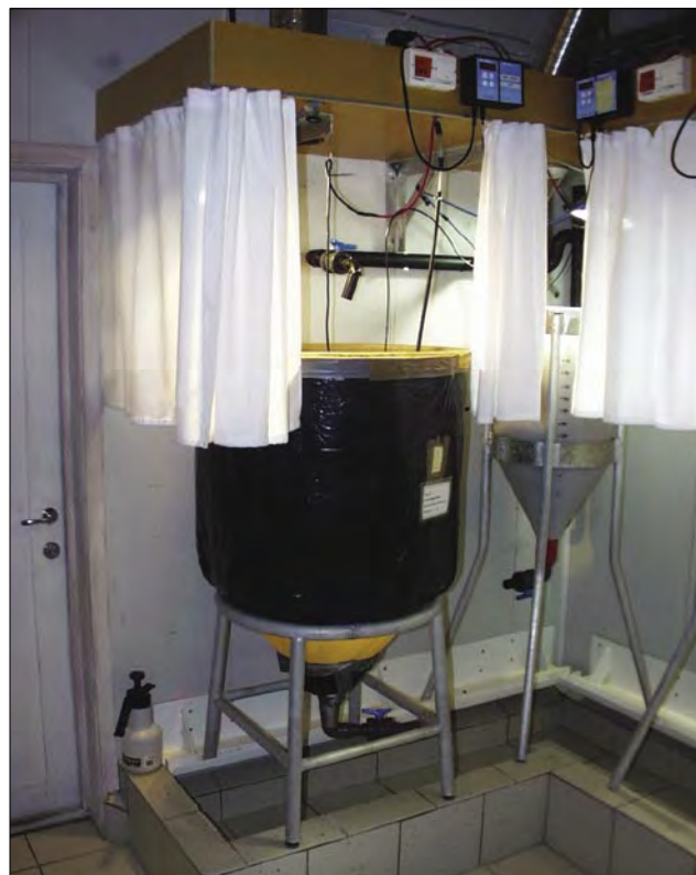
Figur 4 Klekketank for Artemia cyster. Incubator for hatching of Artemia cysts.
