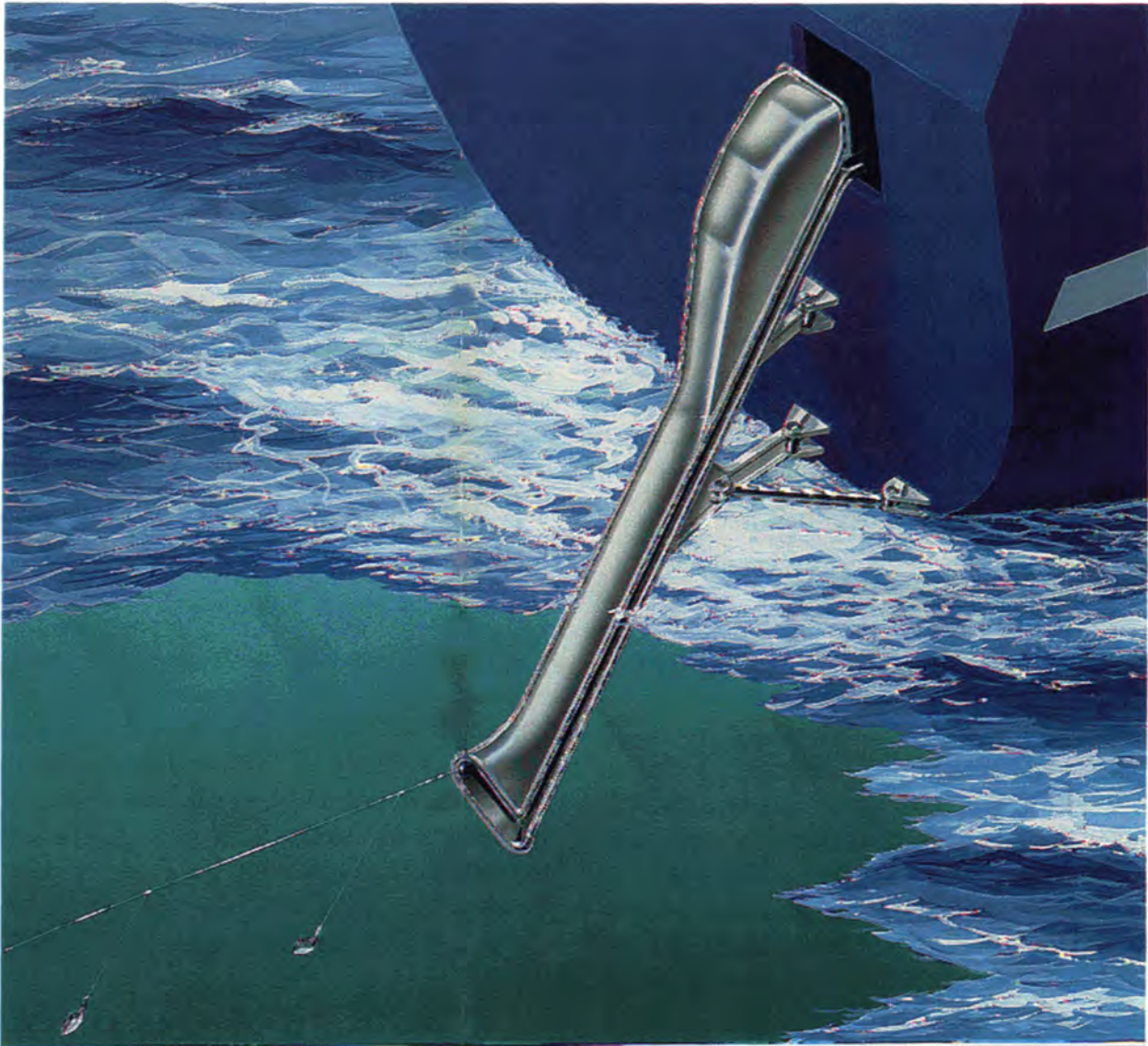
Figur 5.2.2 Setterøret leder lina et stykke ned i sjøen under setting. The setting funnel guides the baited line beneath the sea surface during setting.
