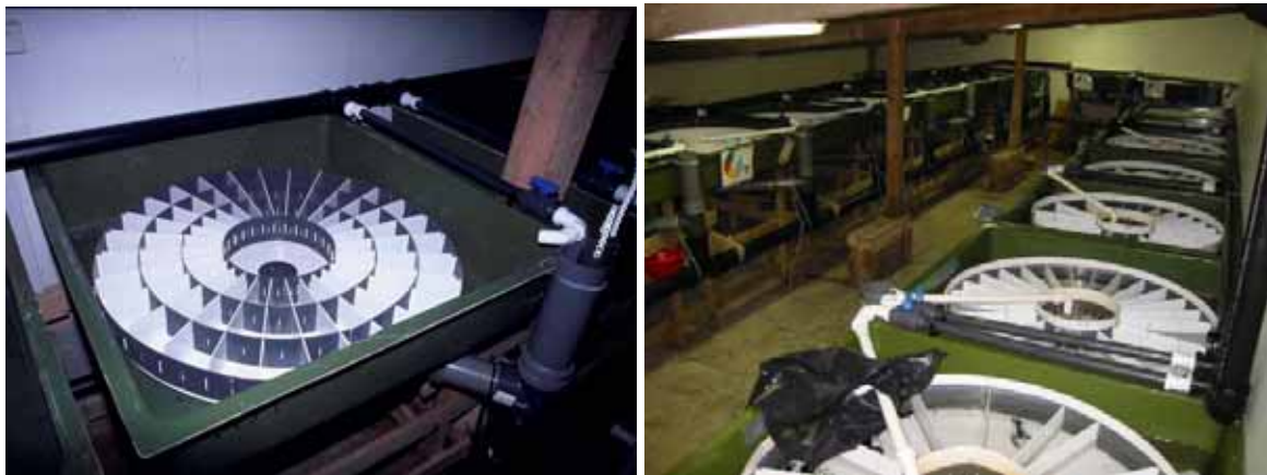
Figure 5.2. The wheels with up to 84 compartments used for the feeding experiments in 2001 and 2002
