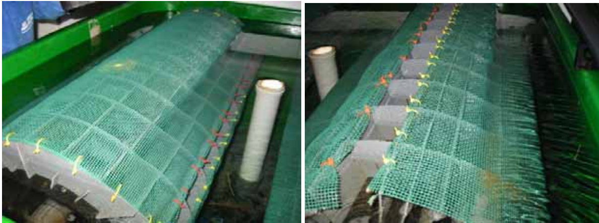
Figure 5.4. Vertical car-o-cells with big compartments (left) and small compartments (right)
