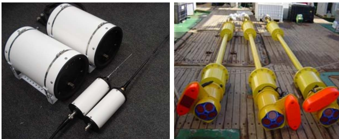
Fig. 2: a) The Remote Echosounder Modules (REMs). b) REM modules have been integrated into multi-frequency echosounder/ADCP buoys
