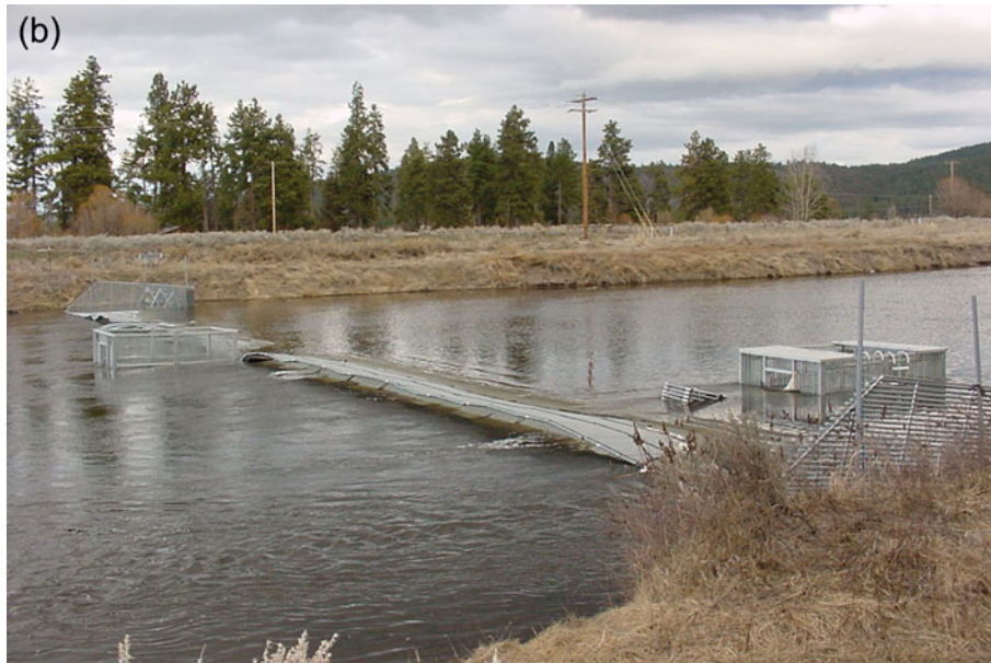
Figure 4b. Photo of complete trap in Williamson River, Oregon (Photographer: J. Anderson).
