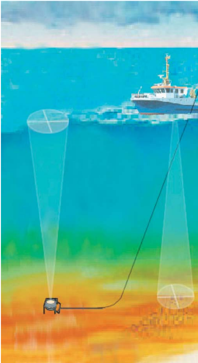
Fig. 1. Survey design illustrating the 38-kHz transducer placed on the sea bottom facing upwards and coupled to the EK500 echosounder onboard the RV Trygve Braarud by cable.
