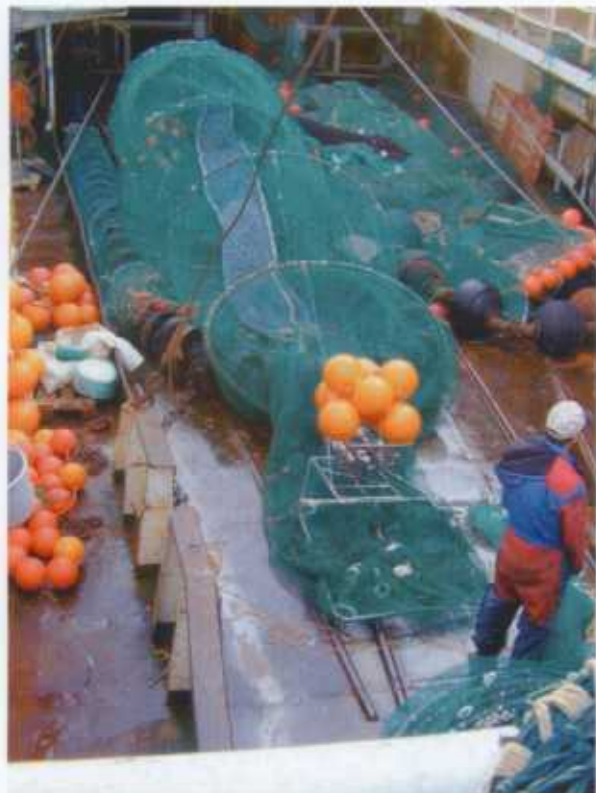
Figure 7. Cod-end with cover cage and acoustic releases on the deck of Myrefisk II
