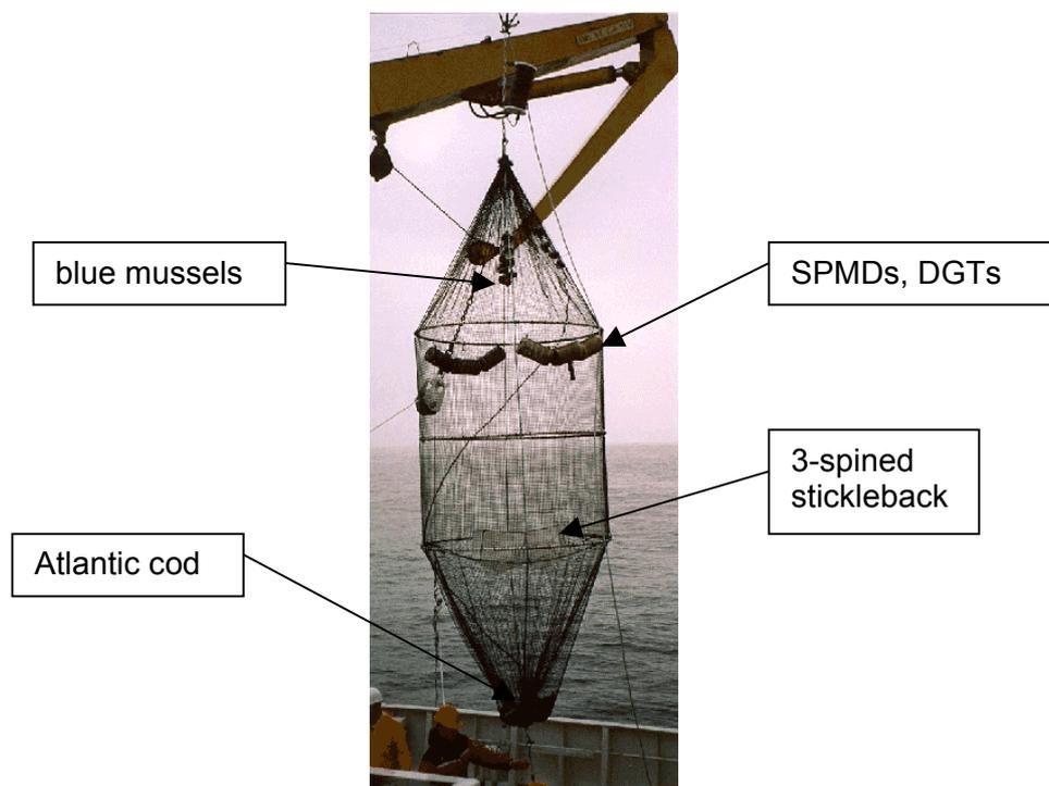
Both cod and blue mussels survived the deployment well, but all stickleback died. Later work has shown that the cage construction was not optimal for the stickleback. For an overview of methods see Table 3.
