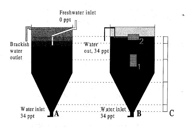
Fig. 1. Silo design and operation principle. Type A with flow-through salinity gradient (incubator 2 and 3). Type B is the traditional silo. Sieve position 1 was operated days - 2 to 3, position 2 days 3 to end of experiment. Freshwater is indicated above position 2. The stacked bars indicate the sectors for larval distribution registrations. A, B and C are in scale. See text for further details.
