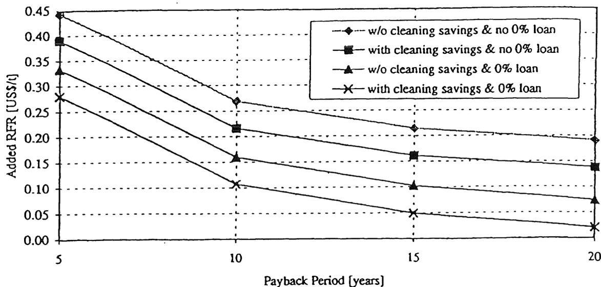
Figure 6. Added Required Freight Rate Required by Ballast Filtration
