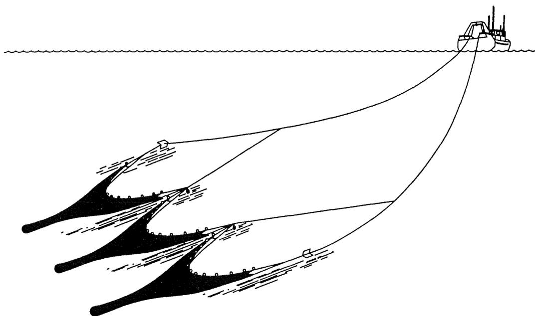
Figure 3. Schematic of triple trawl system
