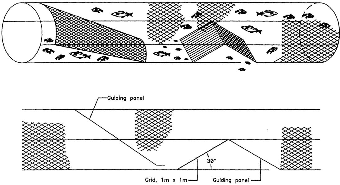
Figure 4. Bottom-mounted grid & extension
