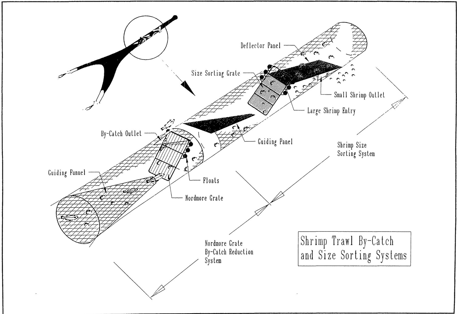
Figure 3: A Diagrammatic Representation of the Size Sorting Grate and its Mechanics.
