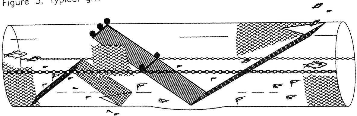
Figure 4. Grid system for releasing small shrimp & small fish
