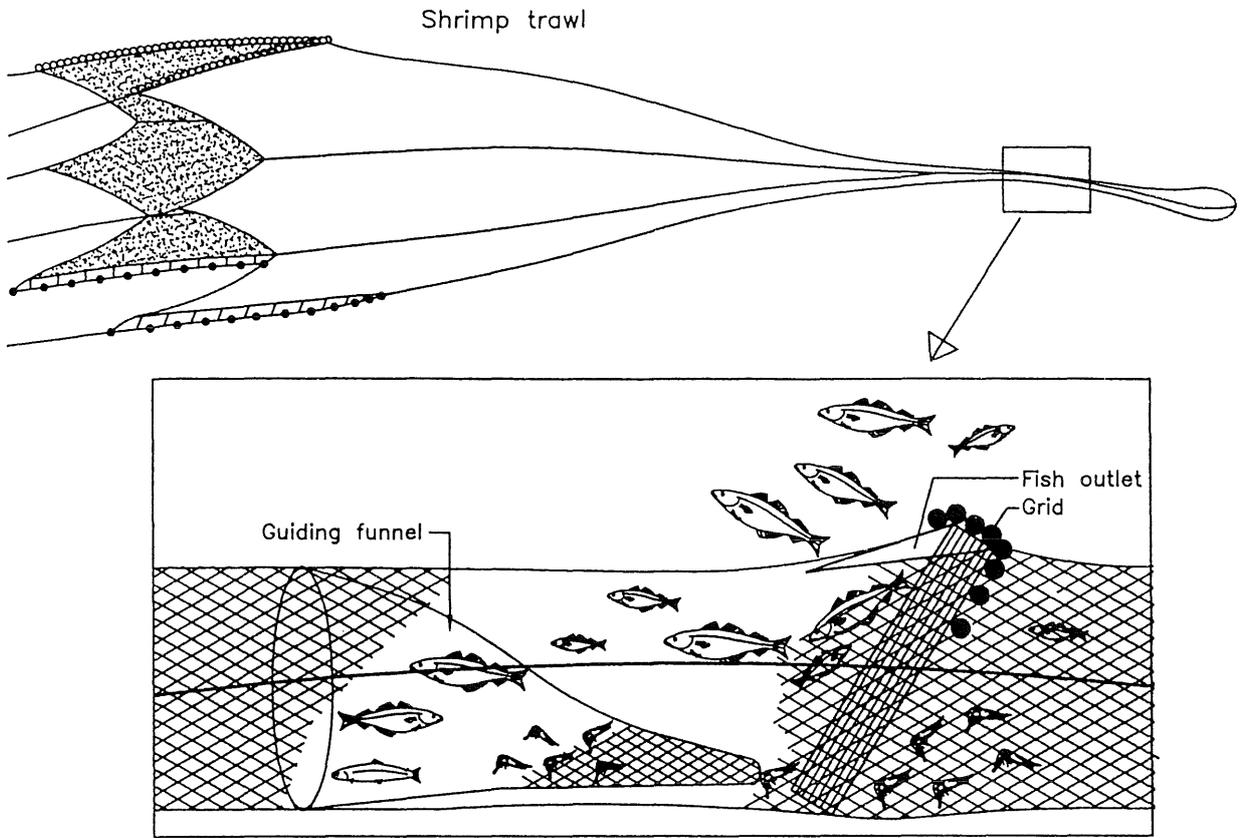
Figure 1. Nordmøre grid shrimp-fish separating system
