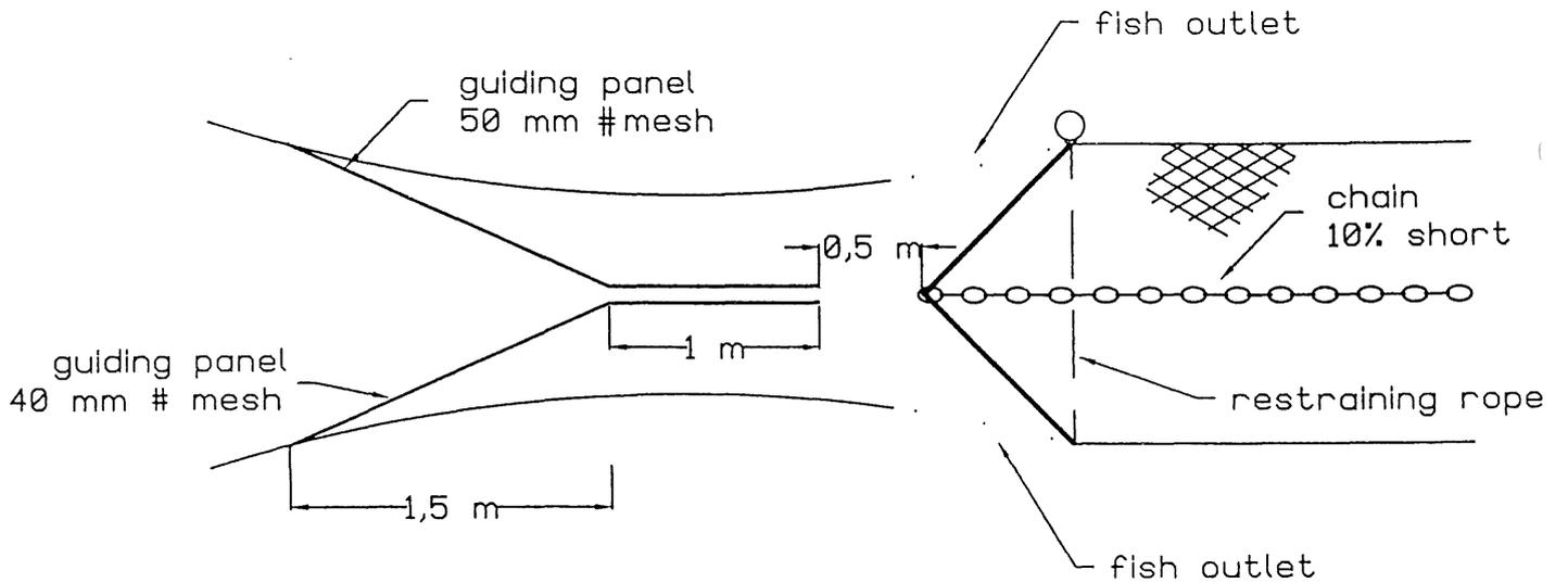
Figure 2. "V-grid" shrimp-fish separating system
