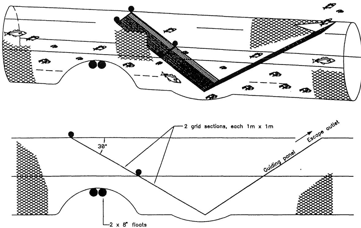
Figure 2. Roof-mounted grid & extension
