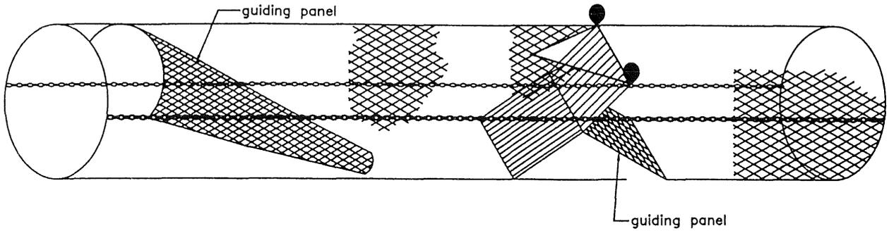
Figure 6. Grid system for releasing small shrimp and all fish
