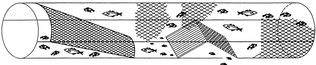
Figure 8. Grid system for releasing small nephrops
