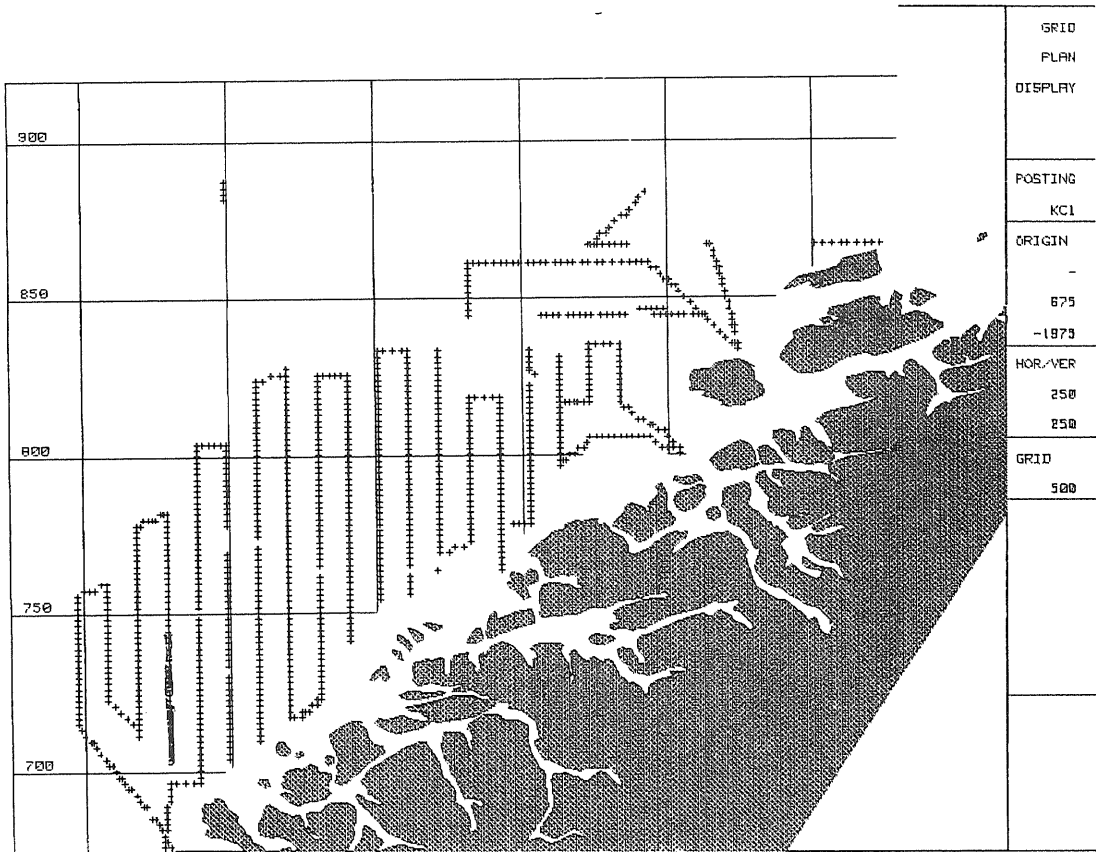
Distribution of survey sample points for acoustic density readings located near Norway. This is for test data file # 4.
