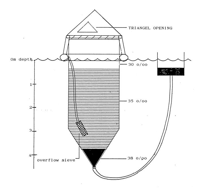
Figure 1. Plastic bag system for rearing of halibut fry.
