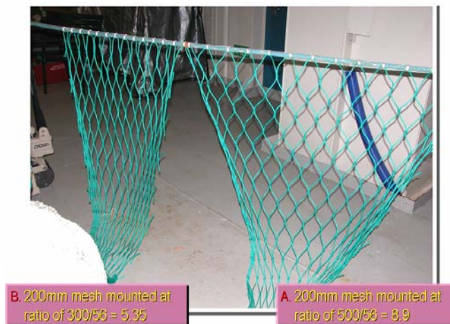
Figure 6.2.2. 200mm mesh mounted at a ratio of 56 meshes per 5m frame rope (Panel A on right of figure); same panel mounted at 56 meshes per 3m frame rope (Panel B on left of figure). The distance between meshes mounted on to the combination in panel A is approximately 9cm with the equivalent for panel B being about 5.4 cm. The lateral stretching in panel A is evident.
