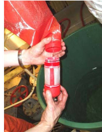
Figure 7 Cod-end may be unscrewed from filtering bag.
