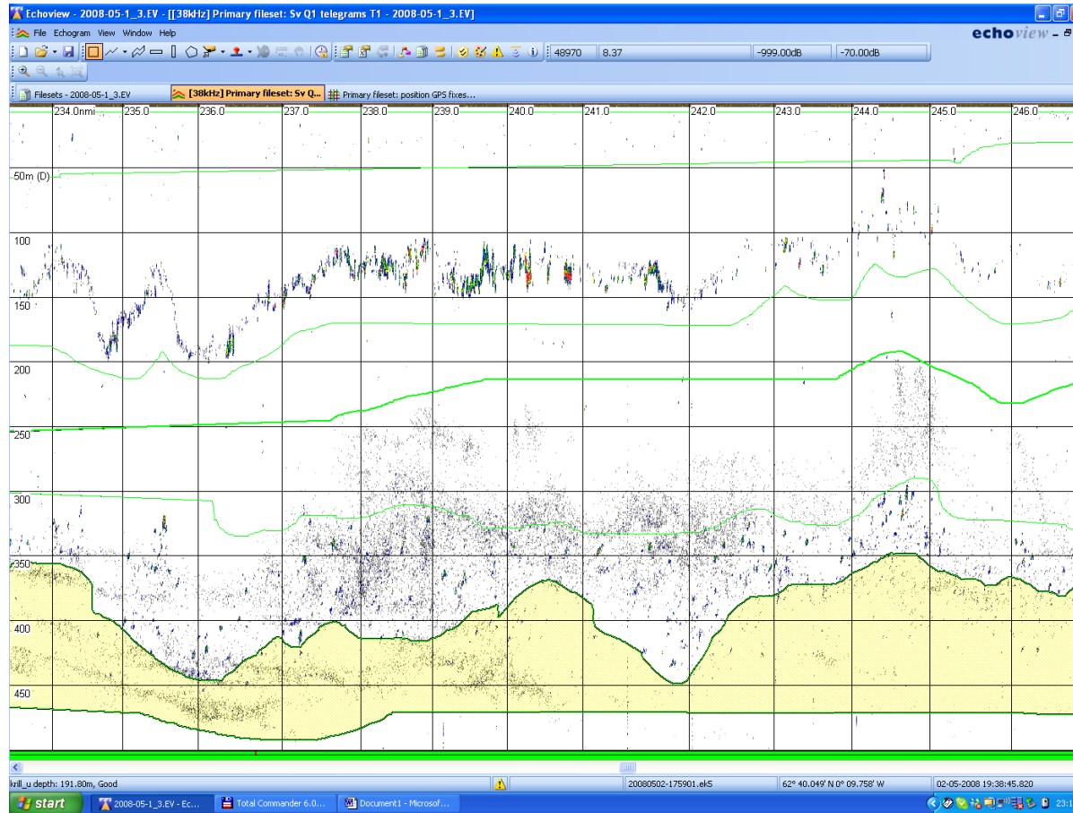
Figure 4a. Acoustic registrations at 62°4 N and 0°15 W in the area around Faroese and EU EEZ. The layer show from top and down: MAC,HER,PLS,KRZ,WHB,KRZ. Thresholding used to detect WHB -69 dB and HER -54 dB.
