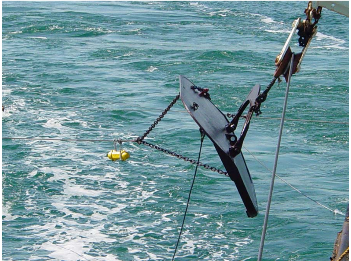
Figure 4.1.2.1. Distance sensors mounted on cable.
