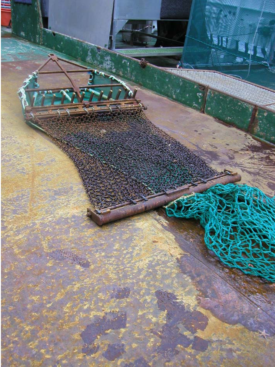
Figure 1b The sandeel dredge, width 1 m.
