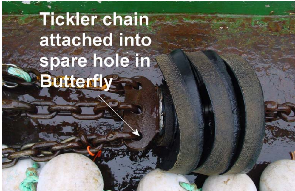
Figure A.3. Tickler chain attachment to the groundgear of the FRS monkfish trawl. Please note to allow ease of handling by Jackson's at the end of the cruises all tickler chains to be removed from the trawls.
