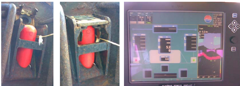
Figure 4.2.6.3.3. SCANMAR instruments on board the Endeavour; connection on the boards (left: open, and middle: closed), and visualization of the recordings in the wheelhouse (right).
