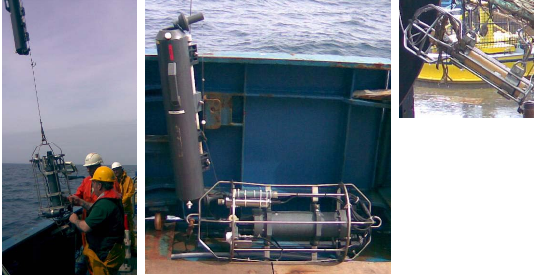
Figure 4.2.6.3.2. CTD deployment on-board the RV Cefas Endeavour during the 3 rd quarter IBTS; left and middle CTD for vertical cast, including the device for taking a water sample, right the mini-CTD that is attached to the GOV net.
