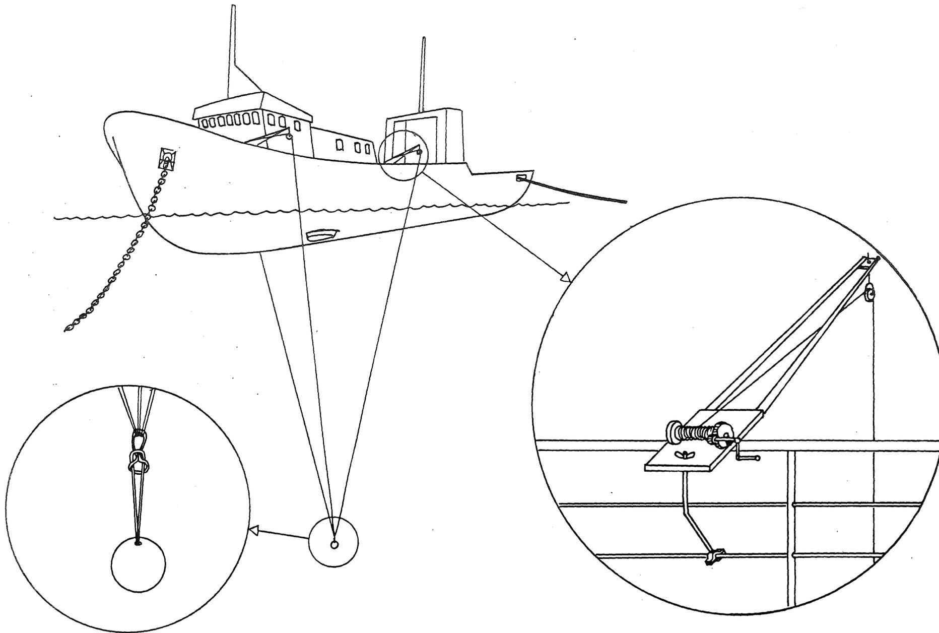
Fig. 4. Measurement configuration and sphere suspension during a calibration exercise.
