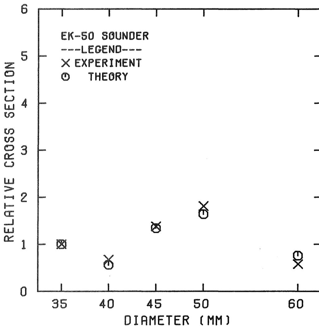
Fig. 1. Comparison of theoretical and experimental backscattering cross sections of copper spheres observed with the EK-50 echo sounder, expressed in normalized units, based on measurements made during the Skogsvaag 1980 experiment.
