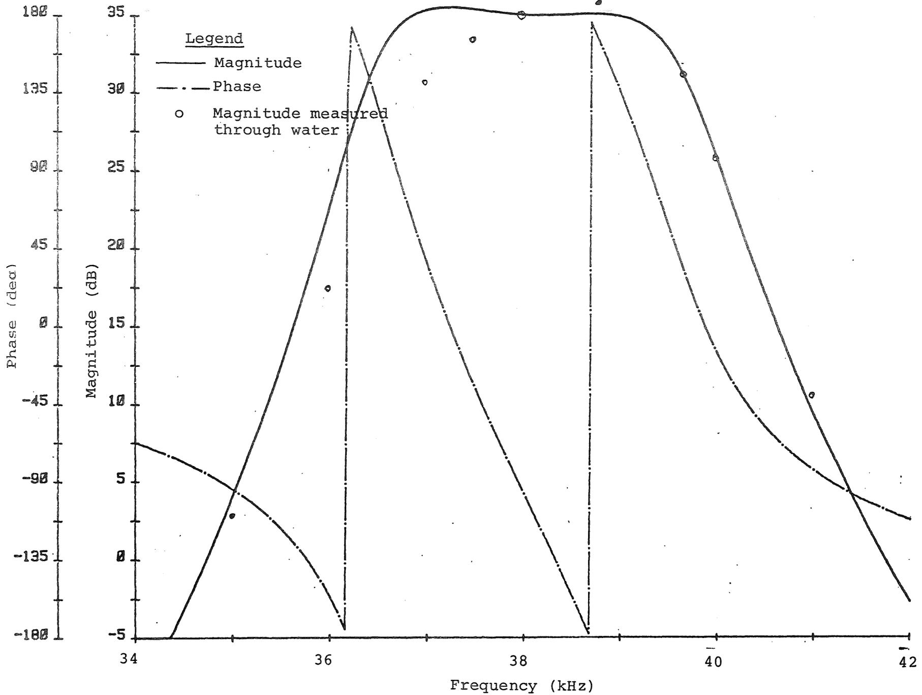
Fig. 2. Measurements of the frequency response function of the 38 kHz unit of the EK-400 echo sounder, made in conjunction with the Skogsvaag 1981 experiment.
