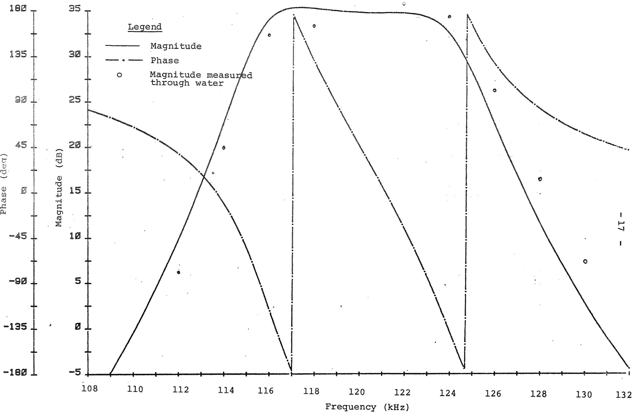
Fig. 3. Measurements of the frequency response function of the 120 kHz unit of the EK-400 echo sounder, made in conjunction with the Skogsvaag 1981 experiment.
