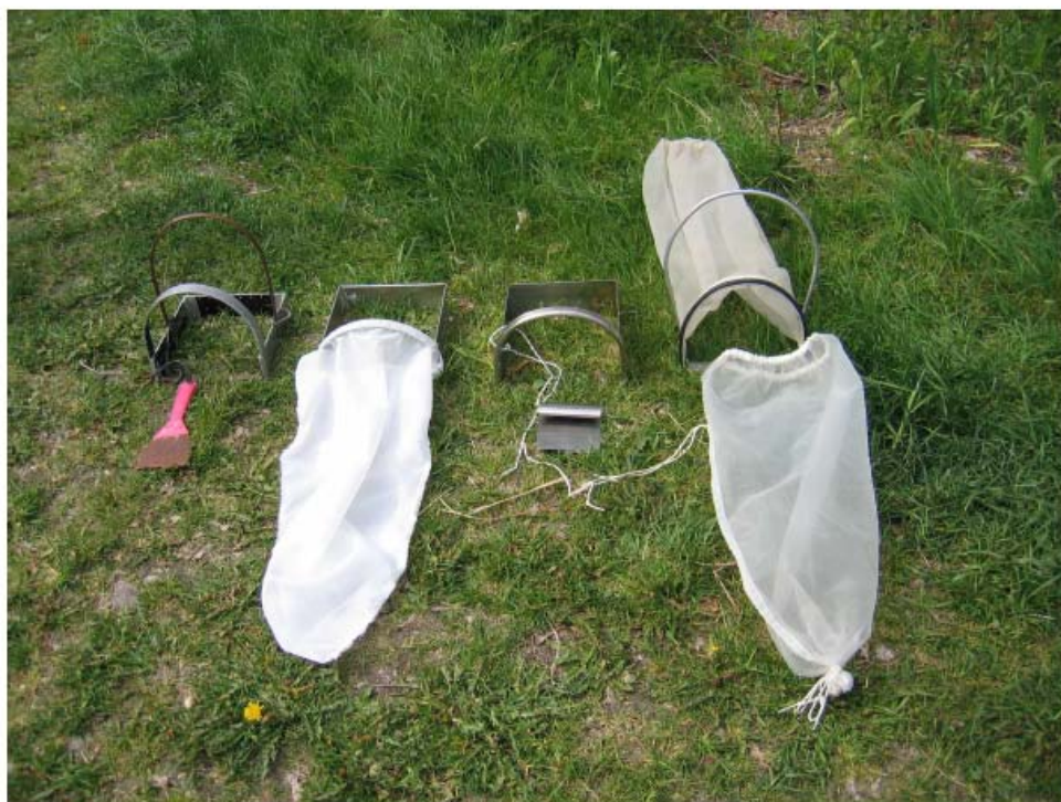
Photo 5. Four different designs of “Kautsky” frame used in different Baltic laboratories (use of this type of frame is suggested by HELCOM COMBINE Guidelines).
