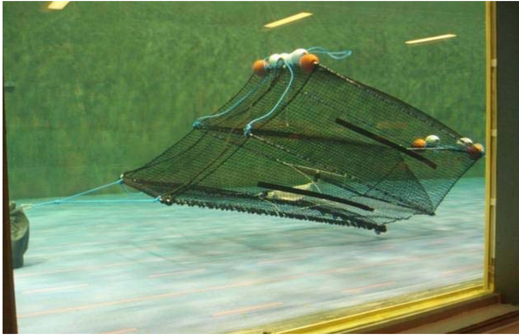
Figure 4.2. The Norwegian two-chamber pot tested in flume tank current.
