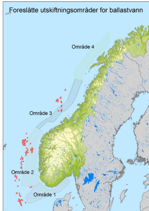
Figure 2. Suggested areas for BW exchange. Area 1 is delimited by Norwegian EEZ towards Denmark. Red dots are permanent oilfield installations. (From Figure 8.1. Dragsund et al , 2007).
