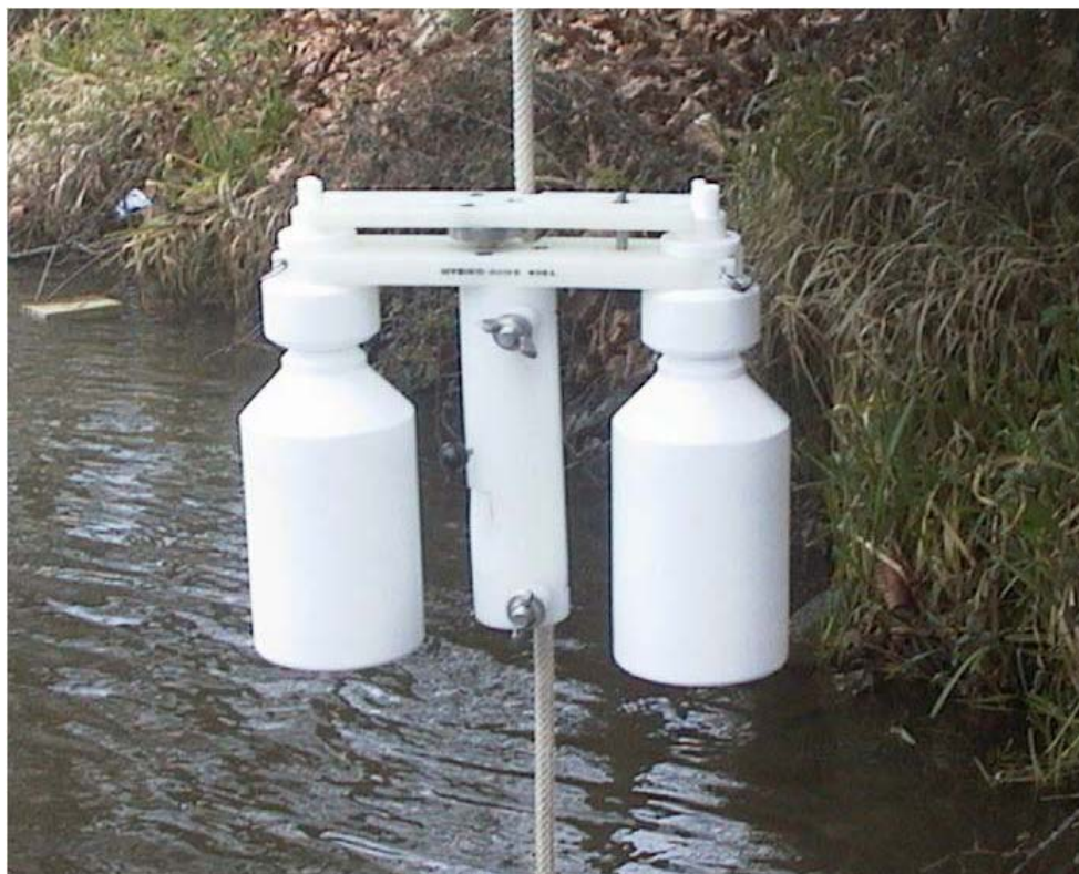
Figure 3. Picture of a MERCOS sampling bottle (IFREMER, France).
