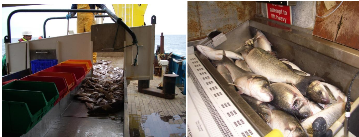
Figure 3: a) fish hopper and sorting table b) workstation with fish bin, and measuring board
