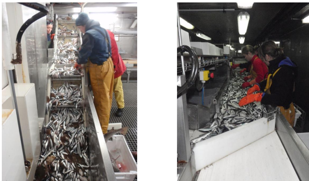
Figure 2: a) Conveyor system from hopper to scales b) Sorting table conveyor system
