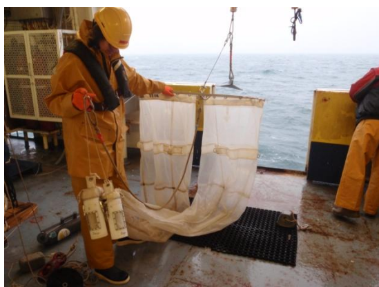
Figure 1: a) Bongo net for zooplankton sampling
