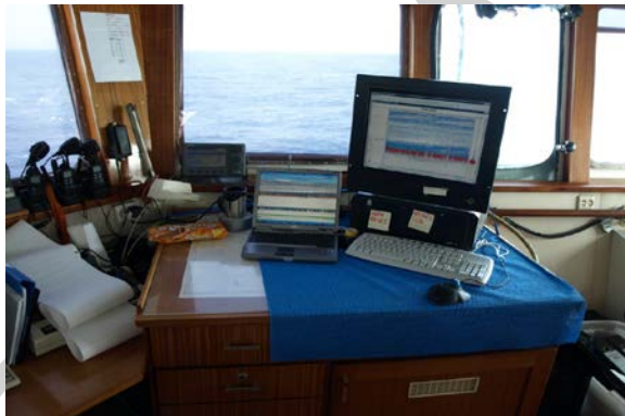
Figure 4. Top side monitoring station located on the bridge. Laptop (left) running Echoview and EK60 topside PC unit (right).
