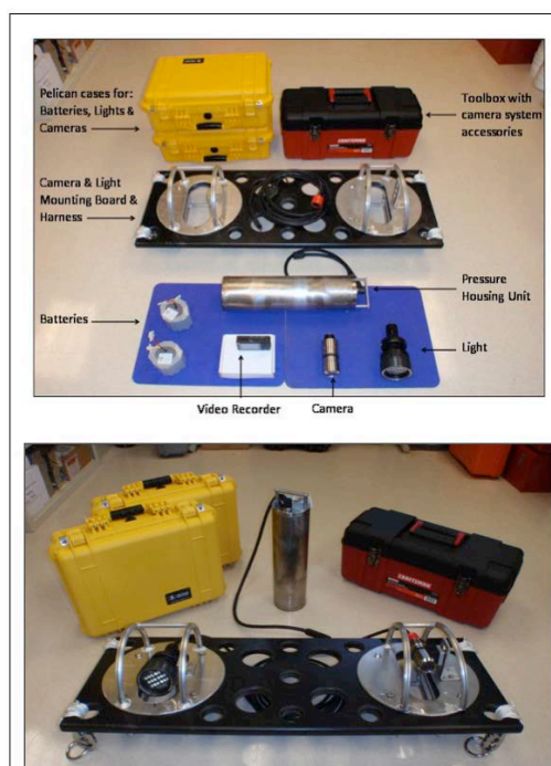
Figure 9. Example of loaner video camera systems currently available to the US Pacific coast fishing industry through NOAA Fisheries NWFSC.
