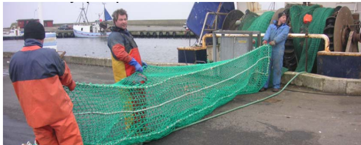
Figure 3. An 8m long square mesh side panel codend.
