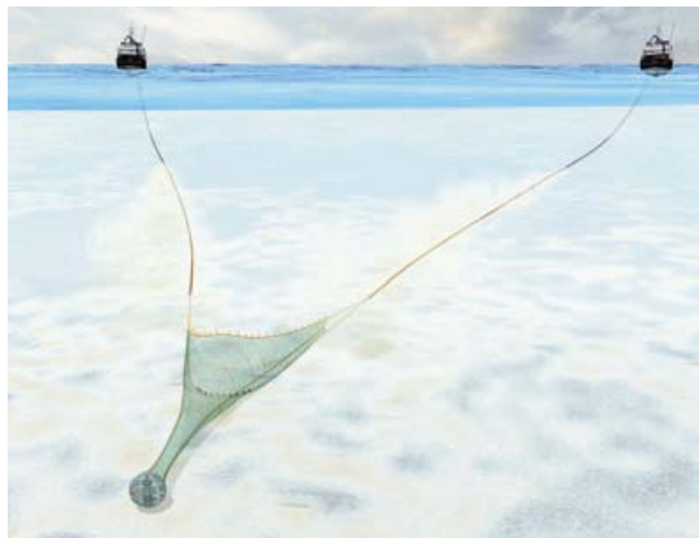
Figure 6. Towing the pair seine demonstrating its similarity to demersal pair trawl. © Crown copyright. Reproduced with the permission of Marine Scotland.
