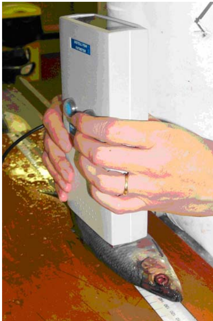
Figure 1: Positioning of the TFFM on herring. Sensor strip is placed below the dorsal fin, along the lateral line. Photos taken from the 2004 lab study.
