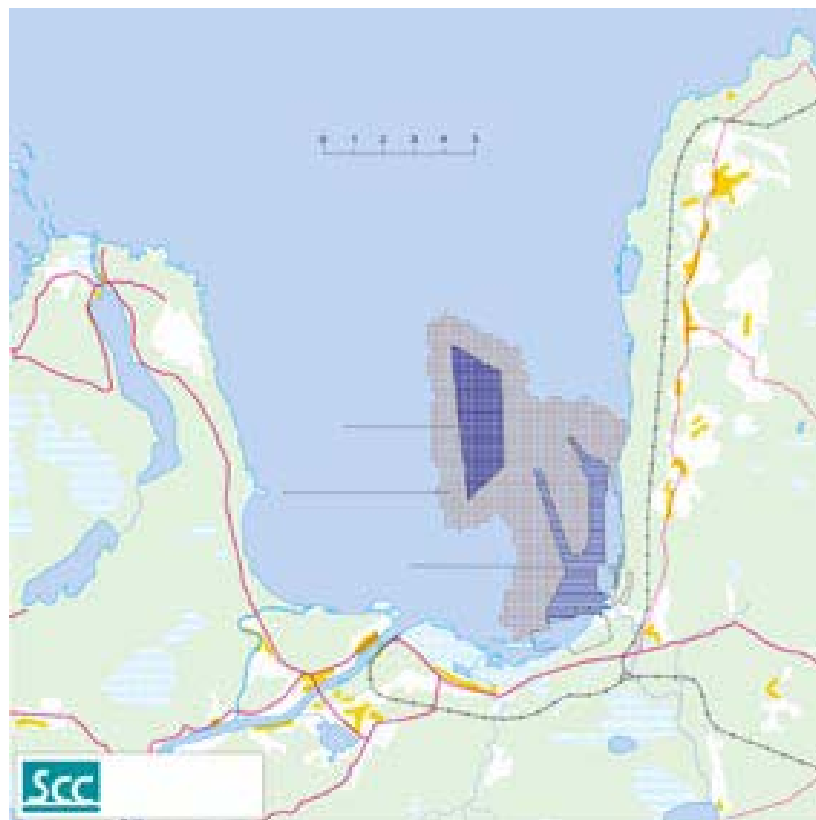
Figure A9.3: Dredging, deposition areas (blue dark) and areas with increased turbidity of water (grey) – at area of construction of Ust-Luga terminal (Project, June 2003).
