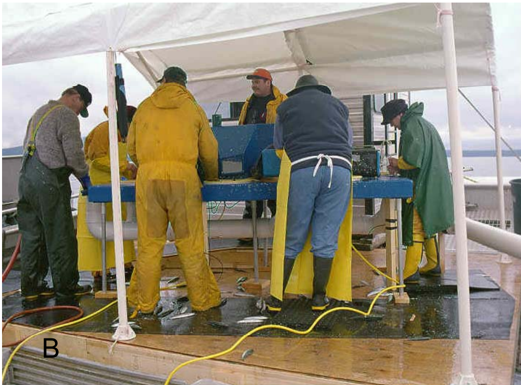
Figure 4 A and B. The tagging table used in 2000 and 2001 is shown with the upper manifold for receiving and distributing dipnets of herring to up to four tagging stations.
