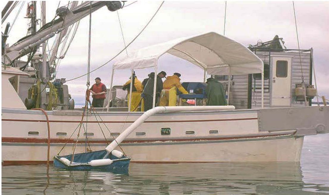
Figure 5. The tagging activities in 2000 and 2001 used a PVC piping system with flowing seawater to direct tagged fish overboard and a recovery pen was used to protect herring from predators.
