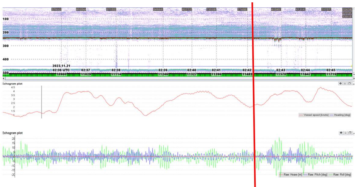
Figure 16 : Performance of the roll/pitch advised controller. The line indicates the change from controller active to inactive.
